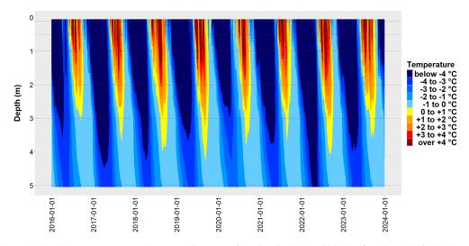
**Figure 6.** The 8-year bedrock temperature record measured at permafrost borehole B2 within the first 5 m (2016–2023). Meter indications refer to the maximum thickness of the permafrost active layer in each summer. Sensor depths are indicated by dotted red lines. Linear interpolation at 0.1 m depth increments was used to model ground temperature between sensors.
